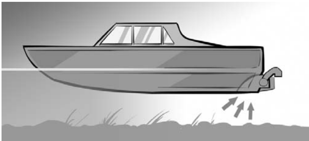
Figure 8. Suction power of the intake
