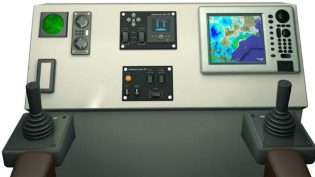
Figure 28. The Alamarin-Jet IO system control panel
